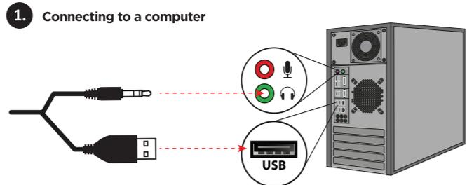
**ATTENTION: background noise appears if the electrical circuit is poorly shielded on the computer. In this case, connect the USB plug to the USB adapter (not included in the package).**
